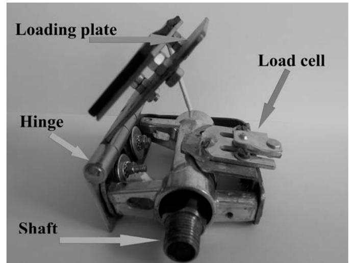
Fig. 1 Pedal – side view
