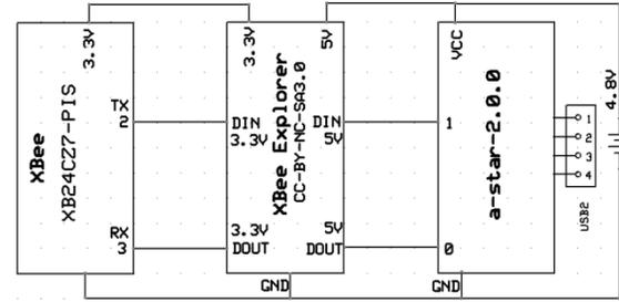
Fig.6Scheme of receiving module
