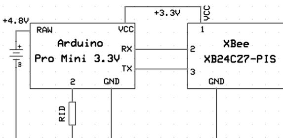
Fig.5Scheme of digital channel
