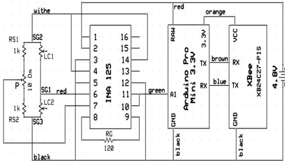
Fig.4 Scheme of one analog channel
